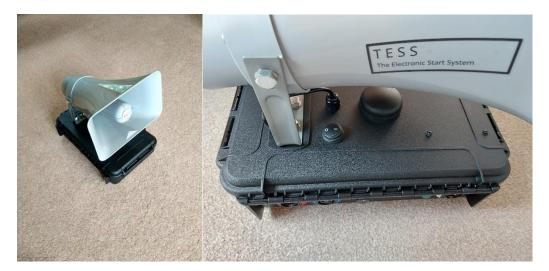
On the left hand side of the unit (looking from the horn "mouth") are a number of connections and controls. To the extreme left is a three pin XLR connector with a RED base. This is to connect to the battery charger which also has a RED XLR connector. Next to the battery charger socket is a BLUE based XLR socket which is for the connection of a Remote Flash Unit.
