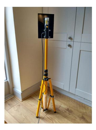
The remote flash takes its trigger pulse from a TESS Sounder Unit. The XLR connector on the remote flash plugs into the BLUE connector on the Sounder Unit.
