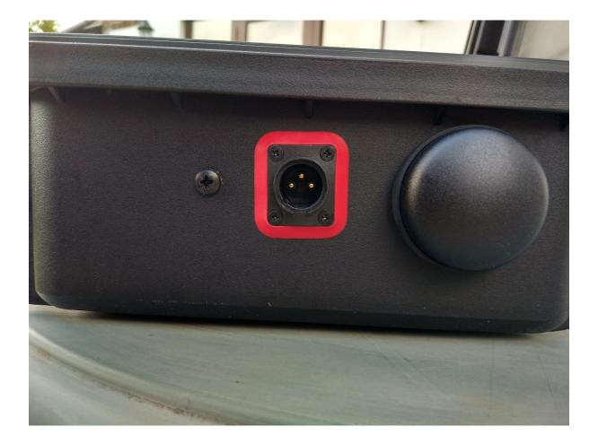
Red for Charger – a three pin XLR connector. The plug on the battery charger goes to this socket.
