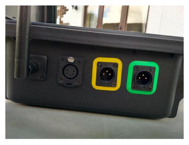
Black – for Start/Flash – a five pin XLR connector. The plug on the Start/Flash actuator connects to this socket.
