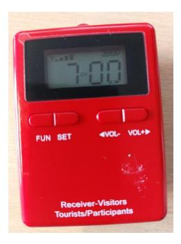
Across the top – to the left is an aerial symbol (like a fork), this shows that a signal is present. Next to the aerial is a signal strength indicator (series of "steps"). To the right is a battery level indicator. These are all similar to the symbols on a mobile 'phone.
